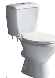
Model: AC2108-B Size: 650x360x690mm WASHDOWN TYPE CLOSE COUPLE PAN VITREOUS CHINA 3/6 DUAL FLUSH CISTERN OUTLET OUTSIDE DIAMMETER 100MM ROUGHING IN WALL TO CENTER OF OUTLET 220MM
