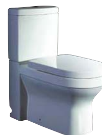
Model: WA101S/SA1010 SEPARATE WASHDOWN WATER CLOSET Size:680x375x790mm Vertical outlet Roughing-in:200mm Water consumption:3/4.5L Diameter of outlet:100mm
