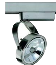
Model: TM202 360° adjustable spot lights, aluminium die-cast body and plastic track adapter, with build-in dimmable electronic transformer, Lamp: QR111 aluminium reflector halogen lamp-max.50w
