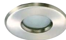
Model: DL401 IP44 Fixed recessed downlights, aluminium die-cast body, reflector and temper glass diffuser, Lamp: MR16 dichroic halogen lamp-max.50w
